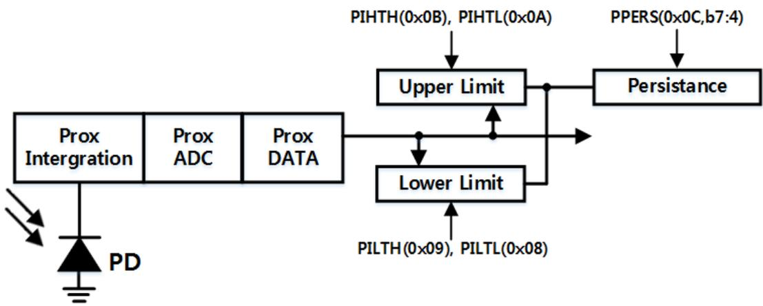
**Figure 3. Programmable Interrupt**
